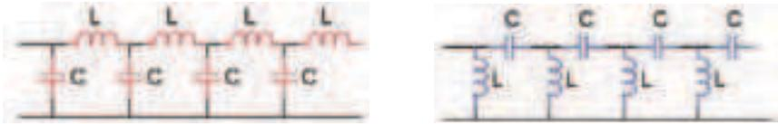
(a) Pure right-handed transmission line (b) Pure left-handed transmission line
